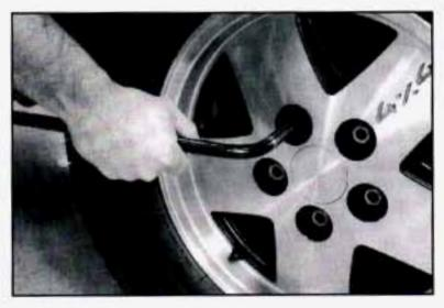
If you have individual wheel nut caps that cover each nut, they must be removed in order to get the wheel nuts. Use the socket end of the wheel wrench to remove the wheel nut caps.
