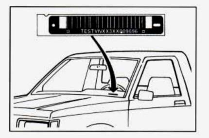
This is the legal identifier for your vehicle. It appears on a plate in the front corner of the instrument panel, on the driver's side. You can see it if you look through the windshield from outside your vehicle. The VIN also appears on the Vehicle Certification and Service Parts labels and the certificates of title and registration.
