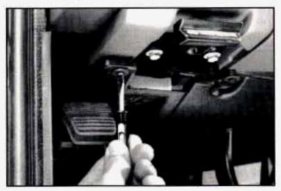
The fuse block is in the instrument panel on the driver's side.
