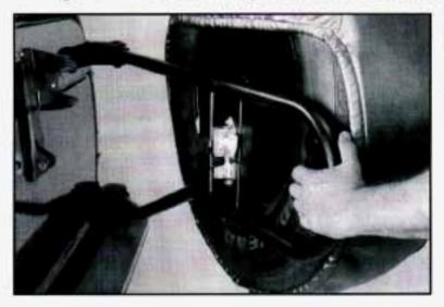
You must move the carrier arm out of the way to open the endgate glass. Here's how to move the arm:
