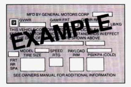
The Certification/Tire label is found on the driver's door lock pillar. The label shows the size of your original tires and the inflation pressures needed to obtain the gross weight capacity of your vehicle. This is called the GVWR (Gross Vehicle Weight Rating). The GVWR includes the weight of the vehicle, all occupants, fuel and cargo.
