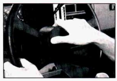
Press the pad in the center of the steering wheel to sound the horn.
