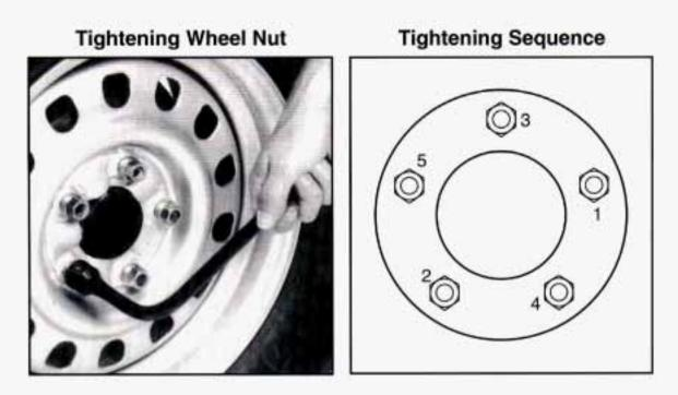
Use the wrench to tighten the wheel nuts firmly in a criss-cross sequence as shown. Remove the wheel blocks.
