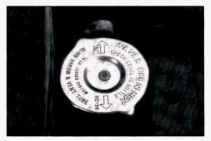
Then replace the pressure cap. At any time during this procedure if coolant begins to flow out of the filler neck, reinstall the pressure cap. Be sure the arrows on pressure cap line up like this.
