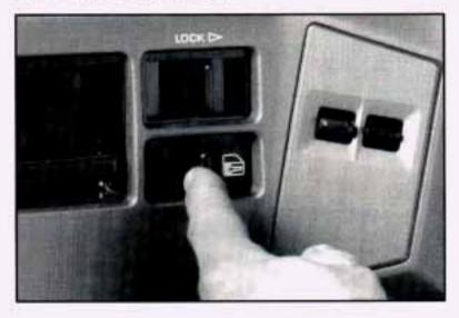
If your vehicle has power door locks, push the power door lock switch on either front door toward the key symbol. This switch will lock all the doors at once.
