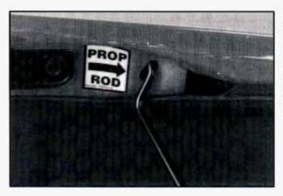
Lift the hood, release the hood prop from its retainer and put the hood prop into the slot in the hood. You may have a light that comes on when you lift the hood.
