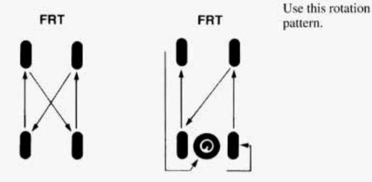
If your vehicle has front tires with different load ratings or tread designs (such as all season vs. on/off road) than the rear tires, don't rotate your tires front to rear.
