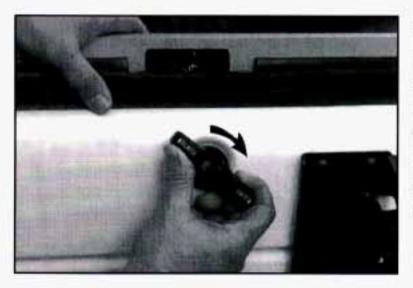
Raise the glass, then turn the lock handle to the right to unlock the endgate. If your vehicle has a endgate-mounted spare tire carrier, you must move the carrier arm out of the way to open the glass.
