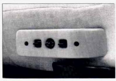
The left control makes the rear of the seat go up and down.
