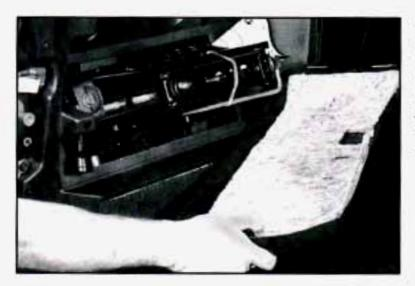
To remove your jack cover on four-door models, pull up on the latch and remove the jack cover. Pull the wheel blocks, jack and wheel wrench off.
