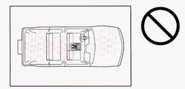
Don't use a child restraint in this position. The restraint won't work properly.
