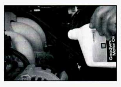
Just fill it enough to put the level somewhere in the proper operating range. Push the dipstick all the way back in when you're through.
