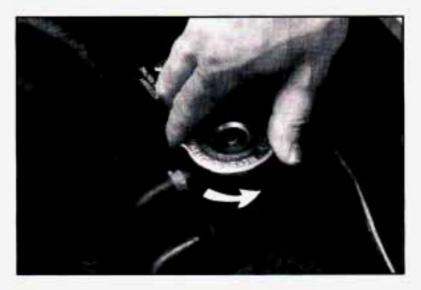
You can remove the radiator pressure cap when the cooling system, including the radiator pressure cap and upper radiator hose, is no longer hot. Turn the pressure cap slowly to the left until it first stops. (Don't press down while turning the pressure cap.)
