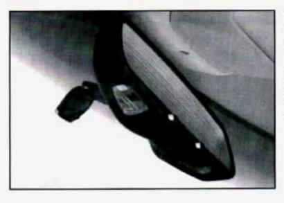
You can also turn the mirror lights on and off by pressing the switch near each light. However, the ignition must be turned to **RUN** or **ACC** for the lights to come on.
