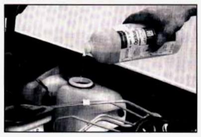
Open the cap labeled "WASHER FLUID ONLY." Add washer fluid until the bottle is full.
