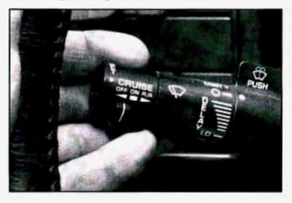
To change the headlights from low beam to high or high to low, pull the turn signal lever all the way toward you. Then release it.
