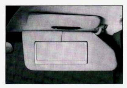
Some visors have a "dual visor" feature where you can swing portions of the visor in different directions at the same time to block out glare.
