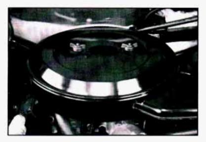
To remove the round air cleaner filter for the 4.3L (VIN Z) engine, turn the wing nuts to the left. Remove the cover and change the filter. Care should be taken during reassembly to ensure that the cover is on straight and the wingnuts are properly tightened.
