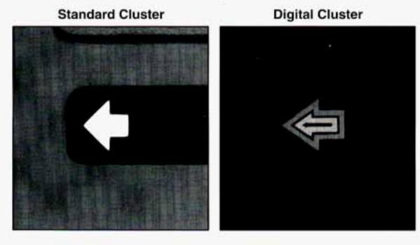
This light with the green arrows is on the instrument cluster. The turn signal indicator will come on whenever you signal a turn or lane change. See "Turn and Lane Change Signal" in this section.
