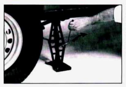
Raise the vehicle by rotating the wheel wrench to the right. Raise the vehicle far enough off the ground so there is enough room for the spare tire to fit.
