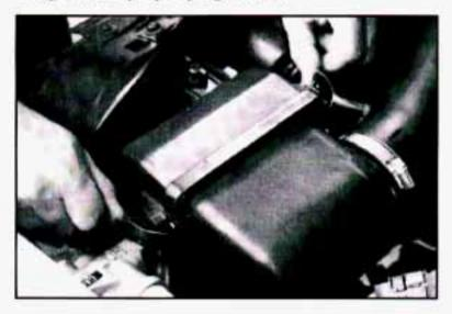
To remove the square air cleaner filter for the 4.3L (VIN W) high performance engine, loosen both wingnuts (one on the duct and one on the cover).
