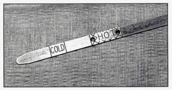
Check both sides of the dipstick, and read the lower level. The fluid level must be in the COLD area for a cold check or in the HOT area or cross-hatched area for a hot check.
