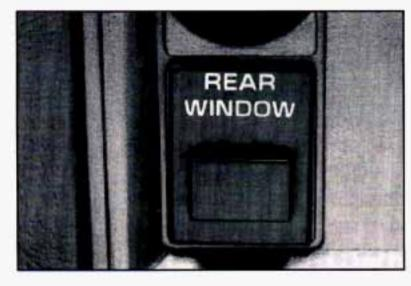
The electric endgate glass release lets you open your endgate glass by just pressing a button. The button is to the left of your radio.
