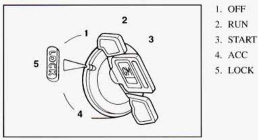
ACC (Accessory): ACC lets you use things like the radio and the windshield wipers when the engine is off. To get into ACC, push in the key and turn it toward you. Your steering wheel will remain locked, just as it was before you inserted the key.
