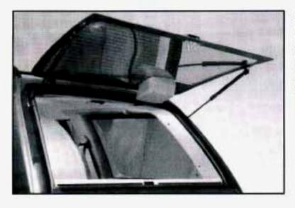
If your vehicle has a endgate-mounted spare tire carrier, you must move the carrier arm out of the way to open the glass.
