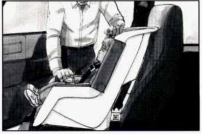
7. Push and pull the child restraint in different directions to be sure it is secure. If you're using a bucket seat, adjust the seat forward until the lap portion of the safety belt holds the restraint firmly. But don't move it any more than needed to tighten the lap belt. To remove the child restraint, just unbuckle the vehicle's safety belt and let it go back all the way.
