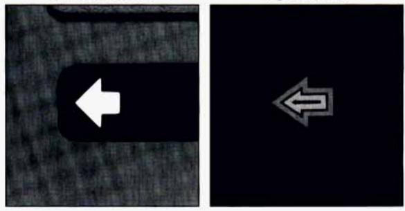
A green arrow on the instrument panel will flash in the direction of the turn or lane change.
