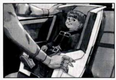
Push and pull the child restraint in different directions to be sure it is secure.
