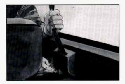
Press the "cinch" button on the retractor cover to set the lock.
