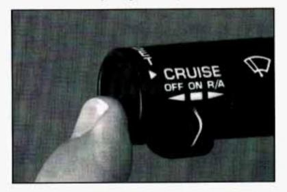
Use the accelerator pedal to get to the higher speed. Push the button at the end of the lever, then release the button and the accelerator pedal. You'll now cruise at the higher speed. Here's the second :
