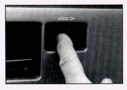
From the inside: To lock the door, slide the lever on your inside door to LOCK.
