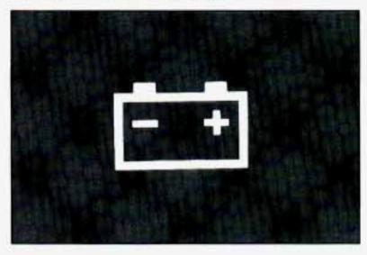
The charging system light is on your instrument cluster and will come on briefly when you turn on the ignition, but the engine is not running, as a check to show you it is working.
