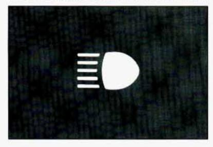
This blue high beam indicator light is on the instrument cluster and is on whenever you use your high beam headlights. For more details about high beams, see "Headlight High-Low Beam Changer" in this section.
