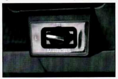
Move the switch to the right or left to choose the mirror, then move the switch from side to side or up and down as needed. If you have the manually adjustable mirror, you can fold it before entering a carwash. To fold, pull the mirrors in towards the vehicle. Push the mirrors back out when finished.
