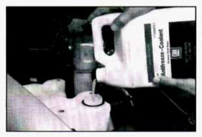
If you need more coolant, add the proper mix at the coolant recovery tank.
