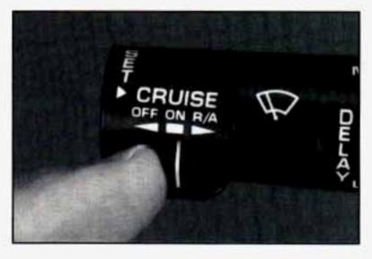
Move the Cruise Control switch to ON.
