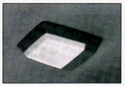
The dome lights will come on when you open the side doors. You can also turn the dome light on by turning the dimmer switch to the right until it clicks.
