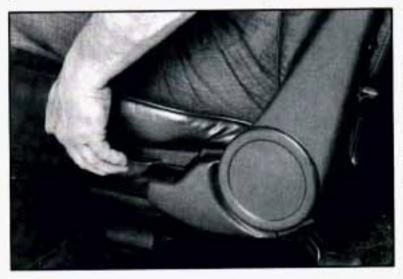
To adjust the seatback, lift the lever on the outer side of the seat. Release the lever to lock the seatback where you want it. Pull up on the lever and the seat will go to an upright position. Don't have a seatback reclined if your vehicle is moving.
