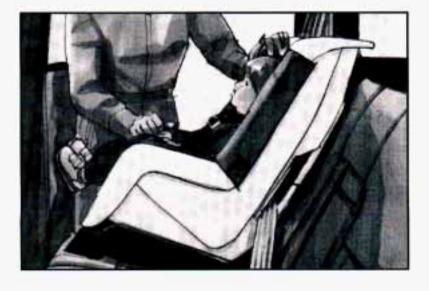
Push and pull the child restraint in different directions to be sure it is secure.
