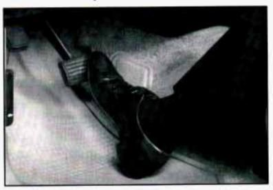
Step lightly on the brake pedal or push the clutch pedal, if you have a manual transmission
