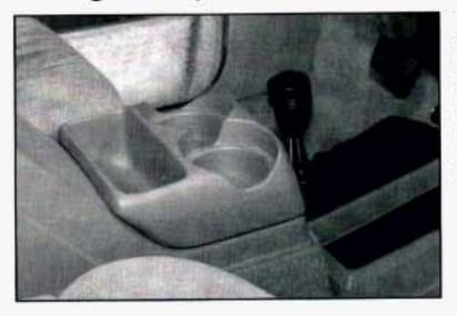
Your vehicle may have a console compartment between the bucket seats. To open it, just lift the top of the console while pressing the button on the driver's side.
