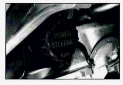
Unscrew the cap and wipe the dipstick with a clean rag. Replace the cap and completely tighten it.
