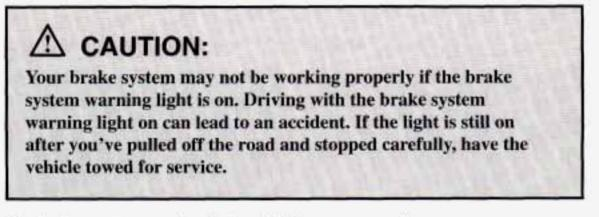
The brake system warning light will also come on when you set your parking brake, and it will stay on if your parking brake doesn't release fully. If it stays on after your parking brake is fully released, it means you have a brake problem.
