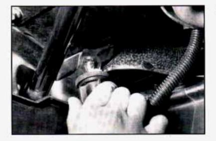
Turn the bulb to the left and pull it out of the socket.
