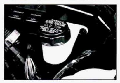
Refer to the Maintenance Schedule to determine how often you should check the fluid level in your clutch master cylinder reservoir and for the proper fluid. See "Owner Checks and Services" and "Recommended Fluids and Lubricants" in the Index.
