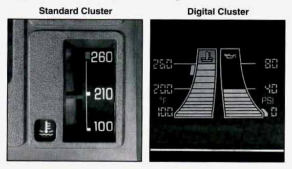
If you have a standard cluster, this gage shows the engine coolant temperature. If the gage pointer moves into the red area, your engine is too hot!
