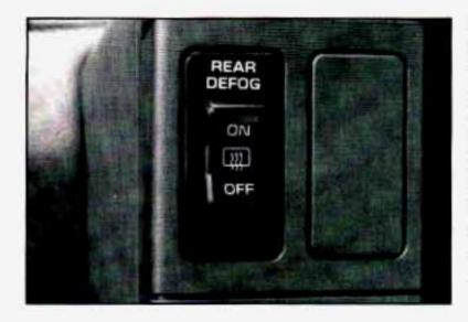
To turn on the rear window defogger, find the switch marked **REAR DEFOG** on your instrument panel. Press "**ON**" until the light in the switch comes on, then release it. The rear window defogger will only work if the ignition switch is turned to **RUN**.
