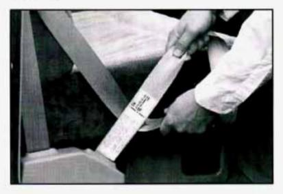
The model number on the replacement belt must be listed on the safety belt you want to replace.
