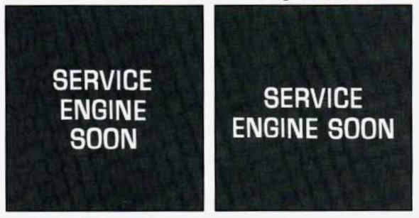
A computer monitors operation of your fuel, ignition and emission control systems. This light should come on when the ignition is on, but the engine is not running, as a check to show you it is working. If it does not come on at all, have it fixed right away. If it stays on, or it comes on while you are driving, the computer is indicating that you have a problem. You should take your vehicle in for service soon.
