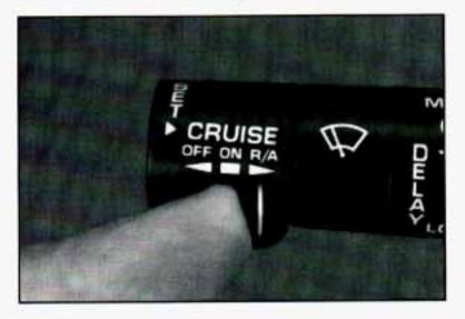
Suppose you set your Cruise Control at a desired speed and then you apply the brake. This, of course, shuts off the Cruise Control. But you don't need to reset it. Once you're going about 25 mph (40 km/h) or more, you can move the Cruise Control switch from **ON** to **R/A** (Resume/Accelerate) for about half a second.
