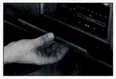
To remove the front ashtray, pull on the front of it and push down at the same time.
