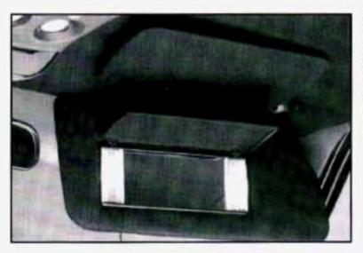
Some visors have mirrors built in, with and without lights. Just lift the mirror cover on each visor to turn the lights on if you have them.
