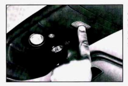
Now, with the compartment door closed, push the button again to make sure the garage door opener operates properly.
