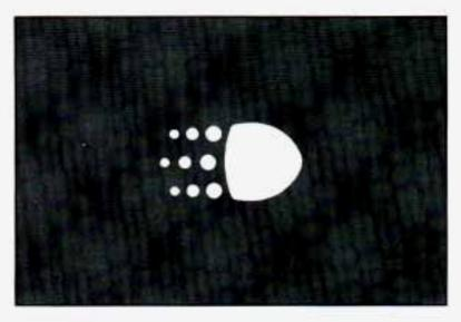
If your vehicle was first sold, when new, in Canada, you will have this light on the instrument panel. It goes on whenever the Daytime Running Lights are on, the ignition is on, the headlamp switch is off, and the parking brake is released.
