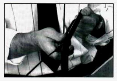
To replace your windshield wiper blade inserts, lift the wiper arm away from the windshield. Pinch the two tabs on the wiper arm and slide the insert out of the blade. Slide the new one in place. Make sure the tabs are locked into position.
