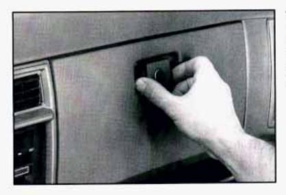
To open your glove box, squeeze the buttons on either side of the keyhole together and pull the door open.
