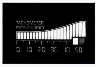
The tachometer displays the engine speed in revolutions per minute (rpm). It is available only with the digital speedometer.
