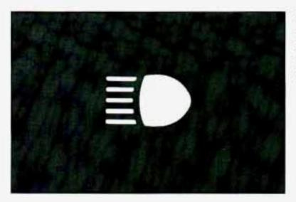
When the high beams are on, this blue indicator light on the instrument panel also will be on.
