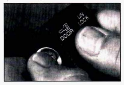
Insert a dime between the two halves of the transmitter housing near the key ring hole.
