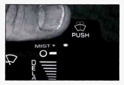
At the top of the multifunction lever there's a paddle marked with the windshield washer symbol and **PUSH**. To spray washer fluid on the windshield, push the paddle.
