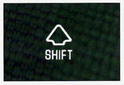
This amber SHIFT indicator light is on the instrument cluster of vehicles with manual transmissions. The SHIFT indicator light will help you get the best fuel economy. See "Shift Indicator Light" in this section.
