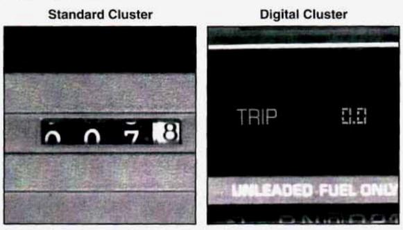
The trip odometer can tell you how far your vehicle has been driven since you last set the trip odometer to zero. Make sure the button is completely depressed to reset the trip odometer.
