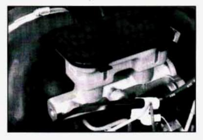
Your brake master cylinder is here. It is filled with DOT-3 brake fluid.
